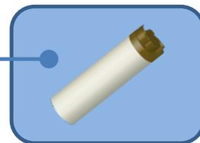
Maximum spinning frequency depends on rotor diameter
